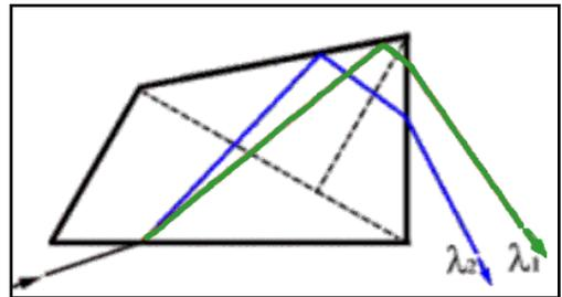
Incident laser beam from an Argon ion laser split into 514nm green and 488nm blue
